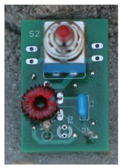
Figure 11. Switch shown mounted on the top side.
