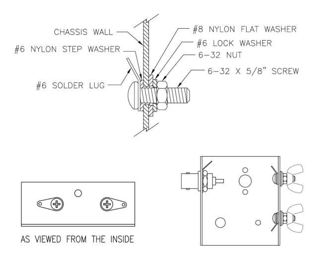
Using the above details, assemble the two antenna connections and the bnc connector to the
