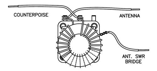
• Cover the back of the poly-varicon with electrical tape. This will act as a surface to secure the toroid. Wire the toroid to the poly-varicon as shown, and solder three pieces of 2" long hook-up wire as shown. We will secure the toroid later with a couple of drops of hotmelt glue or suitable adhesive. Mount the poly-varicon shaft with the screw provided.
