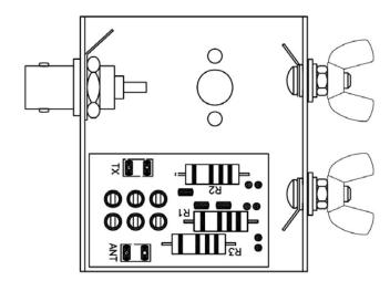
Install the pre-wired Tayloe SWR indicator as shown, and secure it to the chassis with the remaining toggle switch nut.
