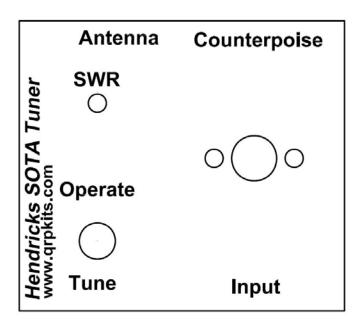
The decals are applied the same as model decals. Cut around each group of text or symbols you wish to apply. It doesn't have to be perfect as the background film is transparent. Apply the decals before you mount anything to the chassis. Use the above picture to get the correct spacing around the holes, as it is very easy to do a great decal installation and have a portion covered up with a knob.
