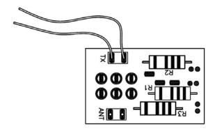
• Pre-wire the Tayloe SWR indicator as shown with 3" long pieces of hook-up wire.
