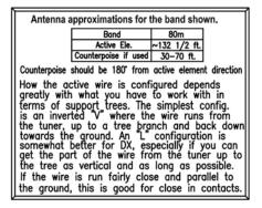
Print out the above label, and scale if necessary to fit the bottom of the chassis. Cover it with a piece of clear packaging tape, and attach it with two-sided tape. The above values are starting points, not absolutes. Your lengths may vary due to many conditions. Some users even omit the counterpoise. Ground conditions, angle of elements in respect to ground, can all affect the overall length. Note what works best for your conditions and make your own chart.
