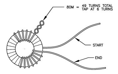
• Wind L1, using T94-2 (red) toroid using the magnet wire supplied to the above specifications and tap at the designated place described above from the "START" end. Remember, every time the wire passes through the center of the toroid, counts as one turn.
