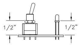
The last component to solder to the Tayloe SWR board is the LED. Use the above dimensions to locate the lip of the LED, and adjust the inside nut of the switch, for the correct fit to the chassis. Then, set the SWR indicator aside, for now.
